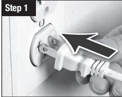
With the power switch in the OFF position, plug the filled humidifier into a polarized 120V outlet. **DO NOT FORCE THE POLARIZED PLUG INTO THE OUTLET;** it will only fit one way. **DO NOT plug in humidifier with wet hands to avoid electric shock.**
