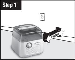
Select a firm, level location at least 6" (15cm) from any walls for proper airflow. Place the humidifier on a water-resistant surface, as water can damage furniture and some flooring.
