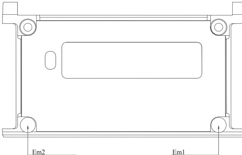
The Em1 and Em2 seals hide the screws that allow to disassemble the calculator-indicator. The sealed cup needs to be dismantled in order to access to the switch that enables to go to the “metrological” mode in order to modify the parameters of the calculator-indicator.
