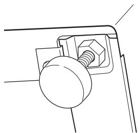
**NOTE:** To minimize vibration, the locking nuts must be tight.
