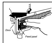
1. **Open the magazine:** pull down down latch and swing door open. Swing magazine cover open.
