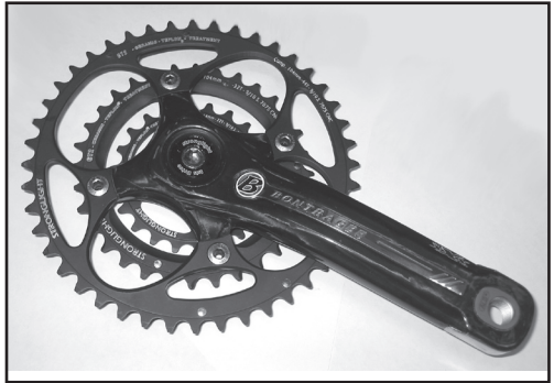
Figure 1- Bontrager Reace XXX Lite carbon fiber crankset
