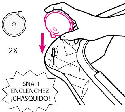
CHECK that casters are securely attached to base by pulling firmly on them.
