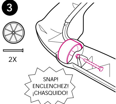
CHECK that wheel pins are held securely in place by plastic tabs.
