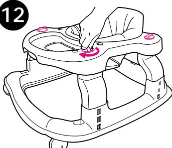
CHECK that bolts are secure by pulling up on tray at four corners.
