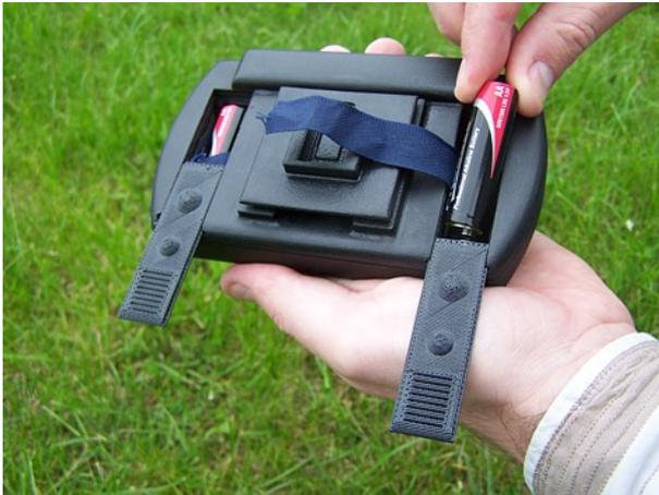
Figure 6.1: Place the batteries into the control unit
