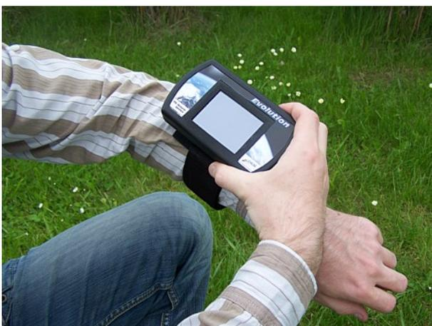
Figure 6.9: Attach control unit at wrist holder (b)
