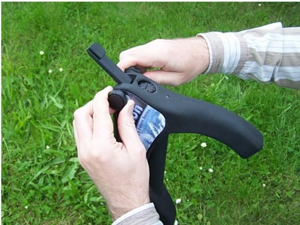
Figure 6.6: Attach control unit at probe (a)
