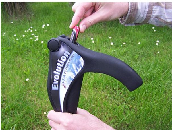
Figure 6.3: Place batteries into the telescopic probe
