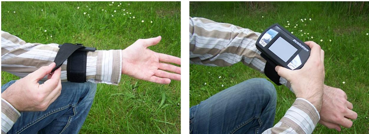
*Figure 5.4: Mounting the control unit to the wrist holder*
