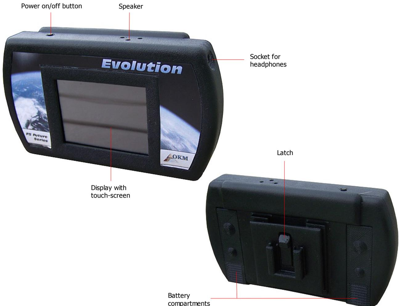
Figure 5.1: Overview of control elements of the control unit
