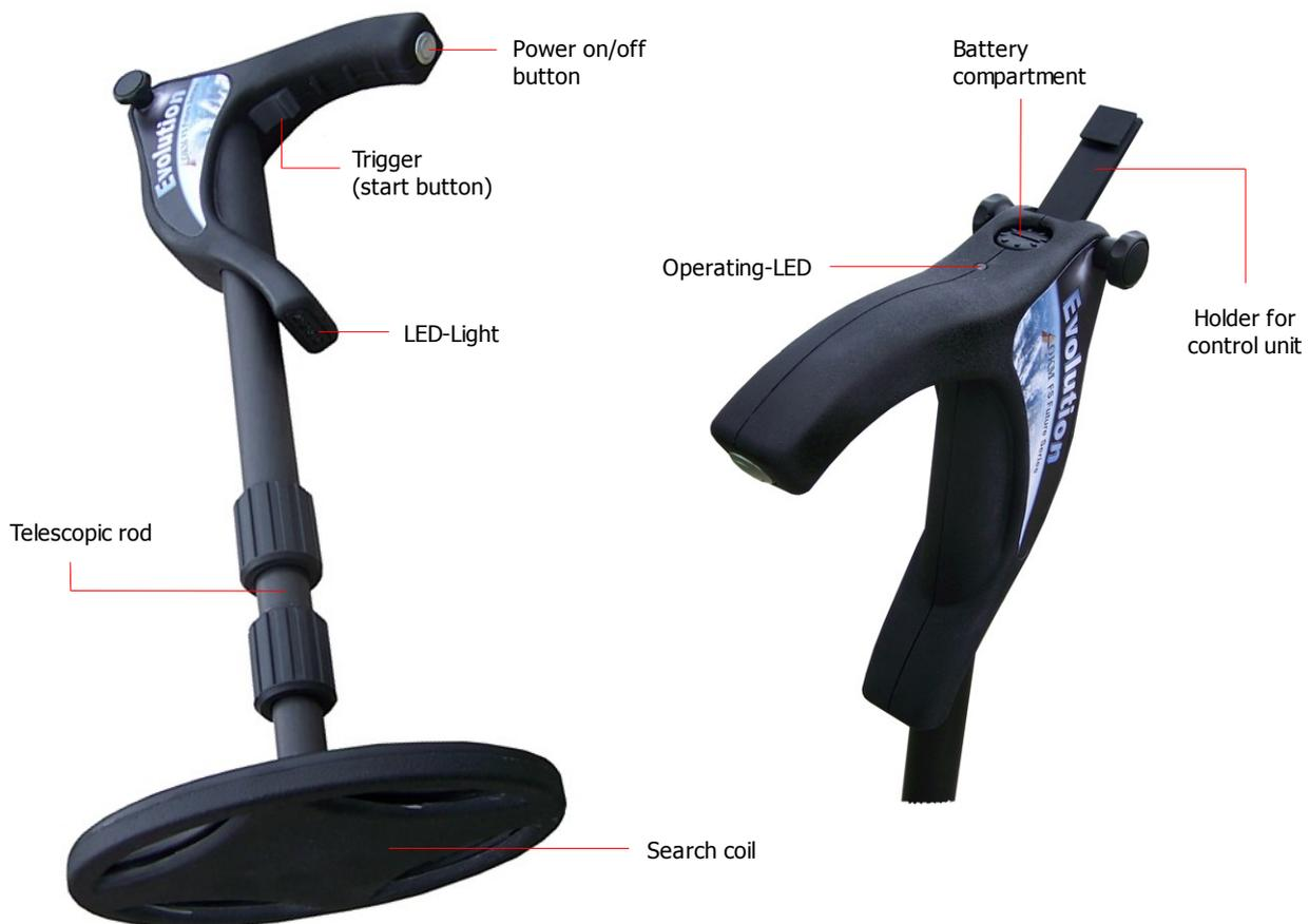
Figure 5.2: Overview of control elements of the telescopic probe
