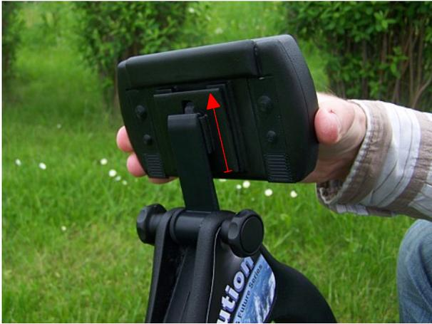
Figure 6.7: Attach control unit at probe (b)
