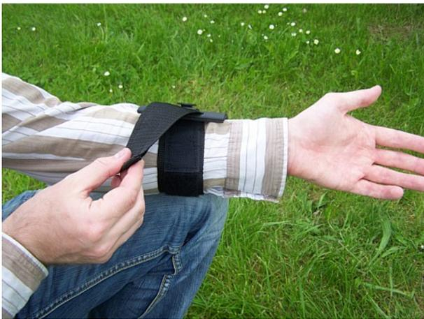
Figure 6.8: Attach control unit at wrist holder (a)
