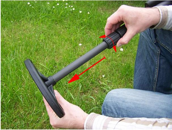
Figure 6.4: Preparing the telescopic probe
