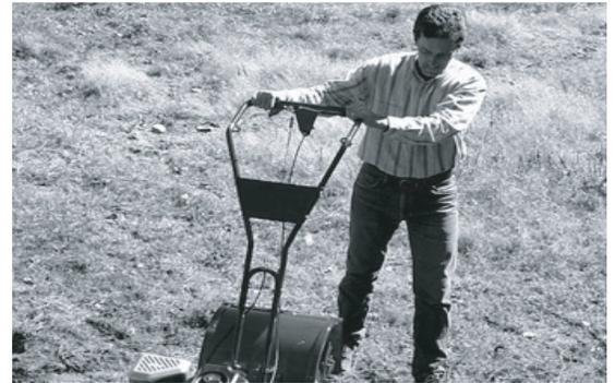
Figure 4-5: With tines out of ground, push handlebars sideways to turn tiller.
