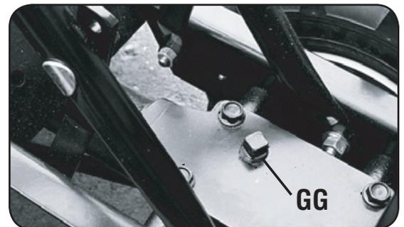
Fig. 2-11: Remove gear oil fill plug.
