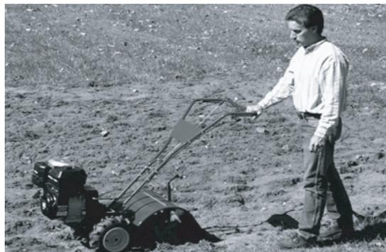
Figure 4-2: Use one hand to guide tiller when moving forward.
