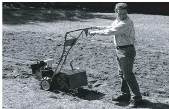
Figure 4-3: Raise tines off ground and look behind when moving in reverse.
