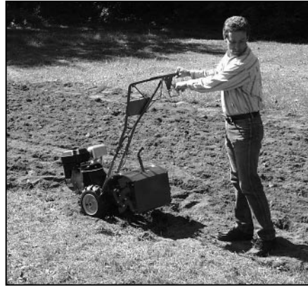
Figure 4-3: Raise tines off ground and look behind when moving in reverse.
