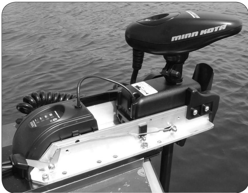
Mount Bracket so that during stow and deploy, the shaft will not encounter boat's rub strip.
