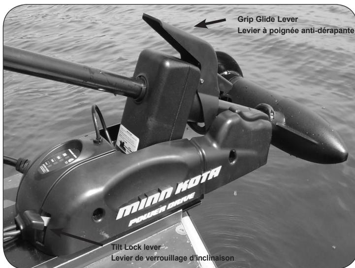
**WARNING : WHEN RAISING OR LOWERING MOTOR, KEEP FINGERS CLEAR OF ALL HINGE AND PIVOT POINTS AND ALL MOVING PARTS.**
