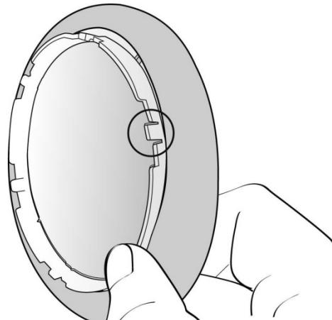
④ In order to optimize the e.ziclean® HOBOT's cleaning performance, place a few drops of your window cleaning solution directly on the pads. Do not wet it too much for fear of it interfering with the device's adhesion to the panel.
