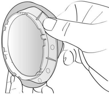
③ Fasten the 2 pad supports under the robot.
