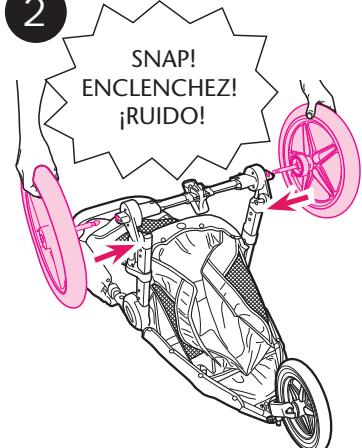
**CHECK** that wheels are securely attached by pulling on wheel assemblies.
