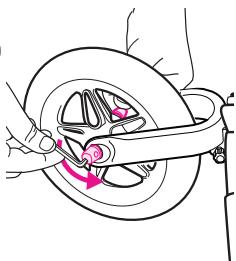
Insert wheel axle **all the way** into front fork slots.
