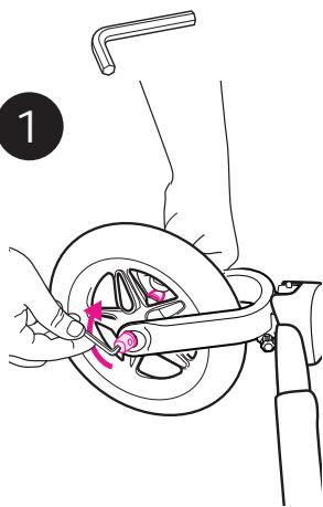
Using 4mm (5/32") hex wrench (not included), loosen axle release nut. Do not remove the nut; the springs may fall out and get lost.
