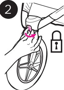
Front swivel wheel locks for use on uneven surfaces such as grass, stones or gravel.
