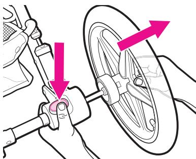
To remove wheel, push button and pull wheel off. Repeat with the other wheel.
