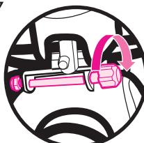
To make the stroller turn more to the right, tighten the screw by turning counter-clockwise.
