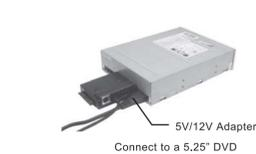
For a 5.25" CD/DVD device, direct plug the SATA Connector or the 40pin connector into the appropriate ports on the rear of the CD/DVD device, and plug the USB signal/data plug (Black) into USB port of PC, then plug the end of the power supply to the 6pin power jack, and the other end plug to power source.
