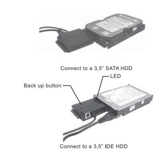
For a 3.5" SATA HDD or a 3.5" IDE HDD, direct plug the SATA Connector or the 40pin connector into the appropriate ports on the rear of the HDD, and plug the USB signal/data plug (Black) into USB port of PC, then plug the end of the power supply to the 6pin power jack, and the other end plug to power source.
