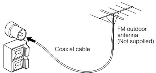
**Using the Coaxial Type Connector (Not Supplied)**
