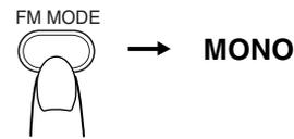
To restore the stereo effect, press the FM MODE button on the Remote Control so that the “MONO” indicator goes off.
