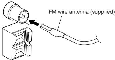
If reception is poor, connect the outdoor antenna.
