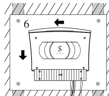
5. Hook the Center Unit onto the attached screws.
