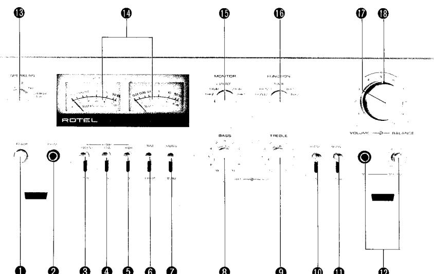
**5 HIGH FILTER** — allows you to reduce high frequency interference whenever you wish to clear annoying record scratches, tape hiss, FM background noise, etc. Normally, however, keep this switch OFF for optimum frequency reproduction of all program sources.
