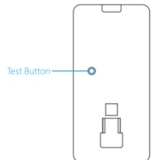
**Testing mode:** After self-testing, press the test button, the sensor enters testing mode, and detects once every 10 seconds. After 3 minutes, the LED flashes twice, and the sensor enters the working mode.
