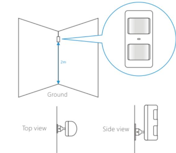
Fix the bracket on the wall with screws and attach the detector to the bracket. Adjust installation height or bracket to change the detection distance and angle. It is recommended to mount it at the height of 2m from the ground.
