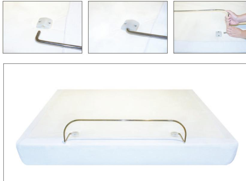
Locate the mattress retainer bar brackets. Slide the left side of the mattress retainer bar into the bracket. Pull the retainer bar to the opposite bracket and secure the right side.
