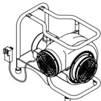
Place blower in a clean fresh air environment. Set blower a minimum of 5 ft. from the manhole opening. *Note: Inspect blower for damaged or worn parts. Inspect all ducting and couplings for possible air leaks prior to blower operation.*
