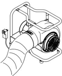
Install duct cuff to exhaust flange and tighten cinch strap. Keep bends and kinks in ducting to a minimum to maximize air flow.
