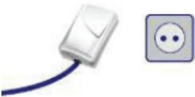
A white powerline Ethernet adapter is shown with a blue Ethernet cable attached, and its power plug is inserted into a standard wall outlet.                 |
