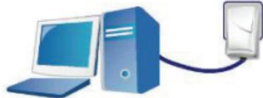
A white powerline Ethernet adapter is connected to a PC tower and a monitor via a blue Ethernet cable. The power adapter is also plugged into a wall outlet. |
