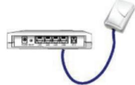
A white powerline Ethernet adapter is connected to a modem via a blue Ethernet cable. The modem is shown in profile with a blue Ethernet port on its side.   |
