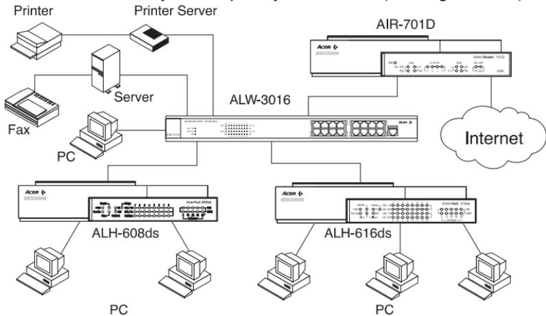
Figure 3-3-1 Application diagram
