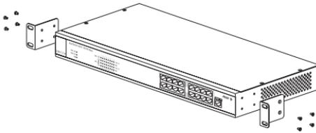
Figure 2-3: Attaching mounting brackets (8 screws: M3x5)
