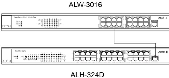
Figure 3-1-1 Connecting to normal port with other hub/switch
