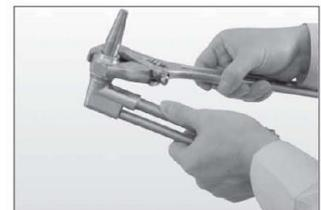
Figure 25, Tightening the Tip Nut
