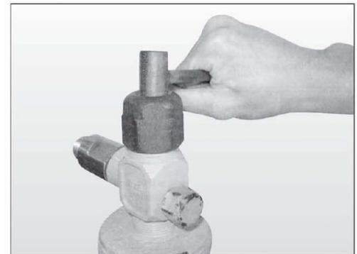
Figure 9, Cracking the Cylinder Valve
