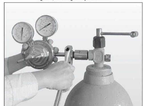
Figure 10, Tightening the Regulator
