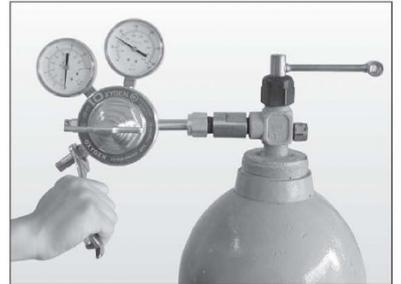
Figure 12, Connecting the Reverse Flow Check Valves
