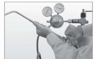
Figure 16, Setting Operating Pressures
