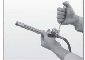
Figure 14, Connecting the Hose to the Torch Handle
