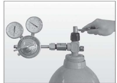
Figure 11, Opening the Cylinder Valve
