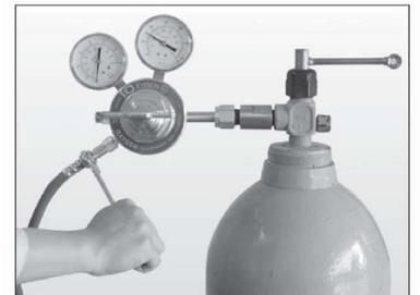
Figure 13, Connecting the Hose
