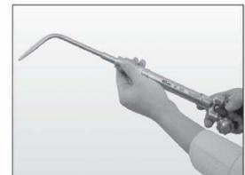
Figure 15, Connecting the Welding Nozzle to Torch Handle
