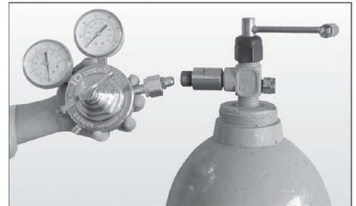
Figure 8, Inspecting the Cylinder and Cylinder Valve
