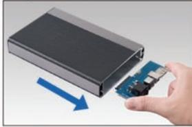
Remove the rear panel and slide out the PCB.
