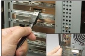
Connect the other end of USB or eSATA connector to the computer.
