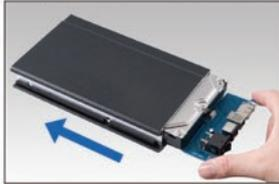
Slide in the hard drive with the PCB back into the enclosure housing.
