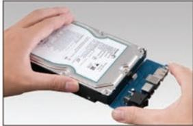
Attach the hard drive to the PCB lining up the pins on the SATA interface.
