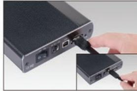
Connect the USB or eSATA cable to the device.
