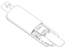
The SIM slot is located at the rear end of the device under a slide out cap
