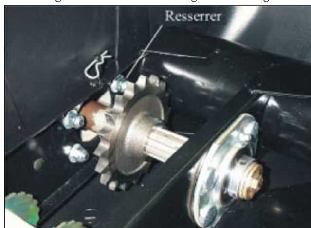
Figure 7-16 Resserrement des boulons
