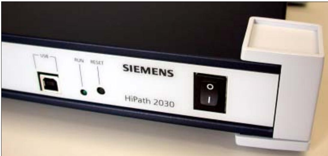
Figure 3-21 HiPath 2020 et HiPath 2030 (photo) – Raccordement USB
