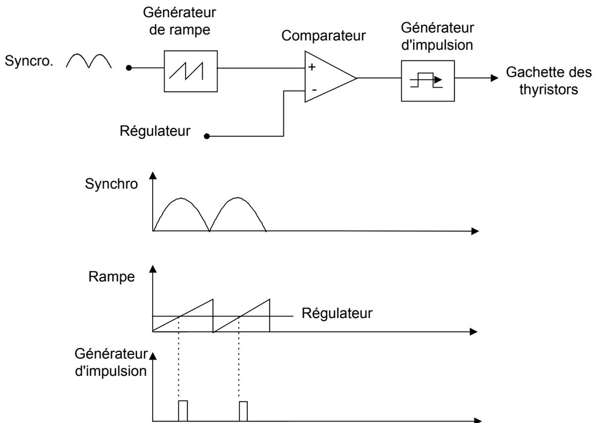
FIGURE 4-13 CIRCUIT D'AMORÇAGE
