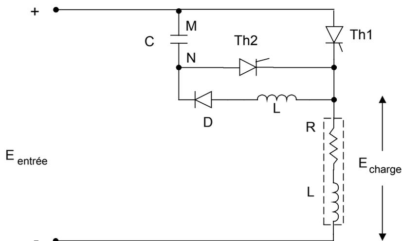
FIGURE 3.4 HACHEUR DÉVOLTEUR AVEC SON CIRCUIT DE DÉSAMORÇAGE
