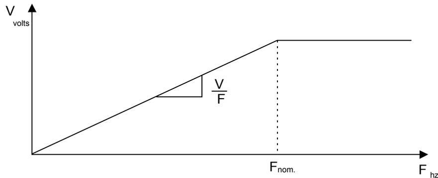
FIGURE 5.14 COURBE TENSION-FRÉQUENCE
