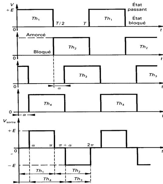
FIGURE 5.9 FORME D'ONDE POR UNE COMMANDE DÉCALÉE
