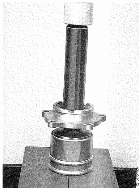
4. Monter le circlips.
