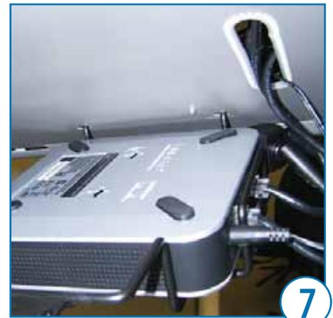
**NOTE:** since the new Router comes with a DC power cord, you should remove the existing DC power cord at this time.
