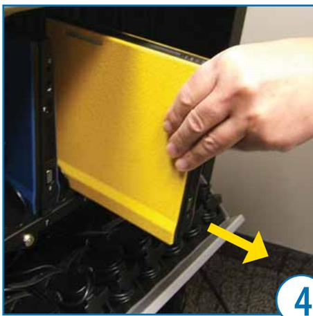
**NOTE:** Each docking station has 3 different Partition types. There are three center Partitions, one right and one left. If replacing a left partition, you will need to pull the docking station forward a few inches in order to access the screw located on the left edge of the dock. Follow appropriate instructions based on Partition type.
