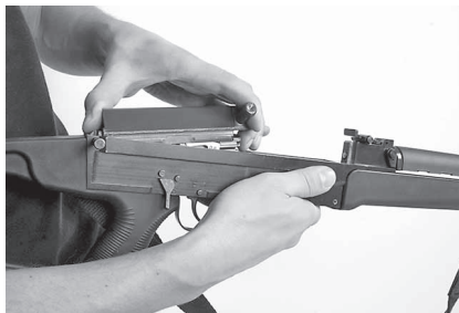
Illustration 29 Taking out the bolt
