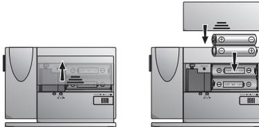
1. Slide the battery compartment cover in the direction of the arrow to remove it.
