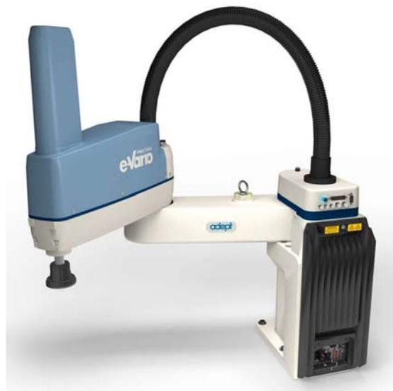
Figure 1.1 : robot Adept Cobra e-Vario 800
