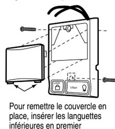
Figure 2 INSTALLATION PRÉ-CÂBLÉE
