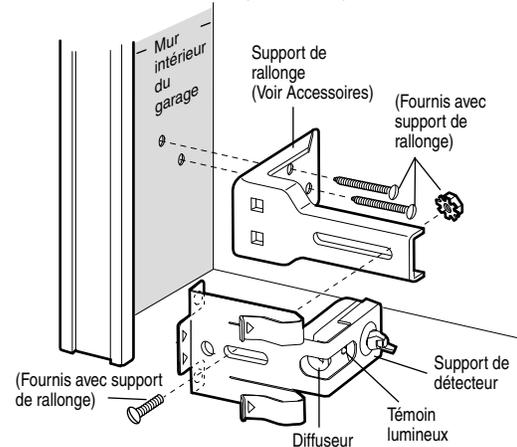
Figure 4 MONTAGE AU SOL (CÔTÉ DROIT)
