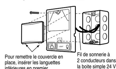
Figure 3 PANNEAU COMMANDE DE PORTE (ARRIÈRE)
