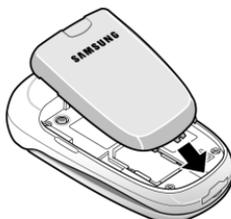
5. Press the battery down until it clicks into place. Make sure that the battery is properly installed before switching on the phone.
