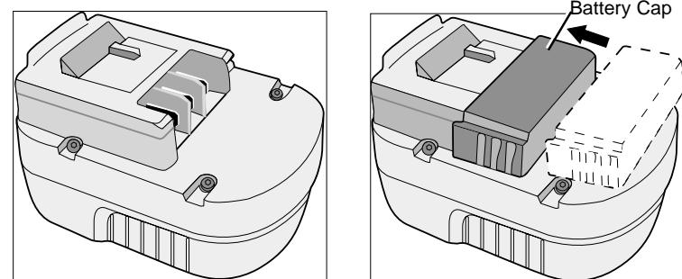
**WARNING!** Do not store or carry battery so that metal objects can contact exposed battery terminals. For example, do not place battery in aprons, pockets, tool boxes, product kit boxes, drawers, etc. with loose nails, screws, keys, etc. without battery cap. Without cap in place, battery could short circuit causing fire or burns or damage to battery.
