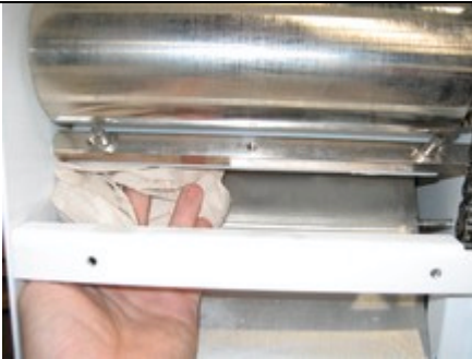
18. Use a soft towel with vegetable oil or shortening to clean scraper and roller on each side.
