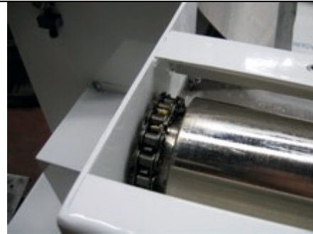
19.1 Add food grade grease over each chain, it may need to be cleaned with a towel if it is dirty before greasing it.
