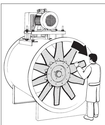
If the fan is delivered without any packing, and if the inlet or outlet are free, it is important to close them with protective plastic film to prevent the entry of dust, foreign bodies, animals, etc ...
