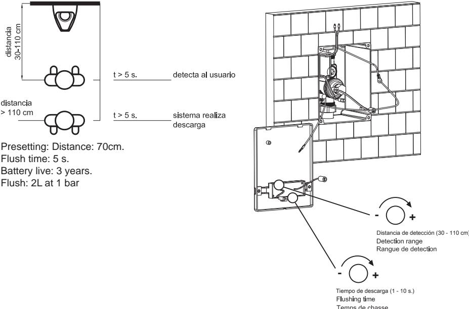
System Works on Infrared Detection principle.
