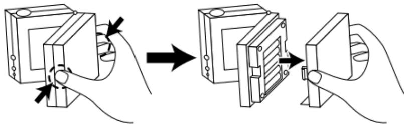
Be sure to match the correct polarity, as shown in the battery compartment. Before you close the lid, press the **RESET** button with the point of a blunt object (such as a ball point pen).
