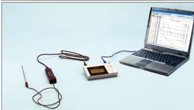
IMAGE 2: CONNEXION D'UN CAPTEUR USB AU PC
