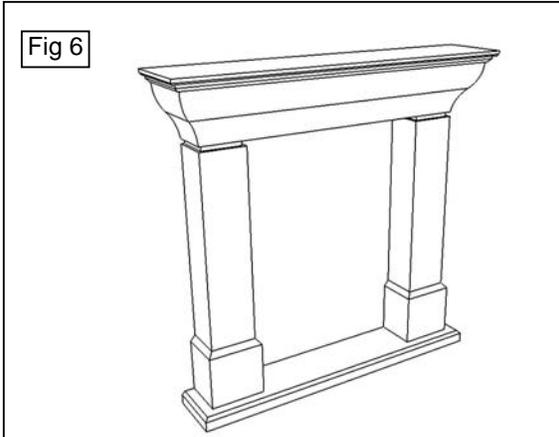
Remove any visual pencil marks with a damp cloth. Using the remaining cement/grout, neaten all joints then wash all residues away with a clean wet sponge. Allow damp patches to dry out before use.
