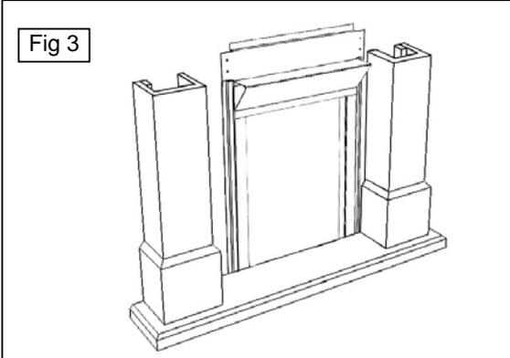
Carefully remove the components individually and return to a 'cushioned' floor. Using appropriate fixings drill and plug the wall central to the hearth and fix both wall brackets with screws provided.
