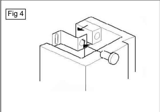
Place a thin line of cement onto the wall and hearth on the inside of the pencilled guideline. Carefully stand leg in position and bed into cement while lining up with the bracket. Push a securing peg through the bracket and into the hole in the block located inside the column leg repeat for second leg.
