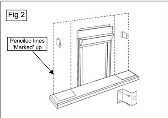
Stand legs onto the hearth aligning with lines and trim kit. Locate blocks that have peg holes inside the column leg (example fig 4) and accurately mark the wall around them for fixing points of brackets. Carefully lift the crossbeam into position and place onto the legs. Centralize and draw pencil lines on wall, around the outside of the surround to aid exact placement later.
