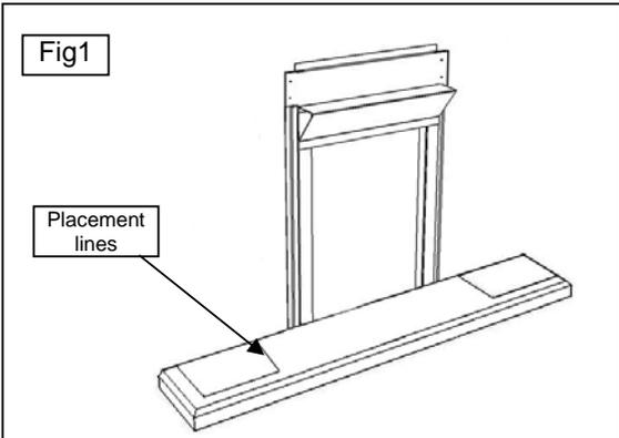
For installation of engine trim kit, refer to trim kit instructions. Bed hearth firmly into position using a mixture of cement provided. Mix a third of the cement at a time. Ensure hearth is central and level to the appliance. For your assistance the hearth has been pre-marked (lined) with a template showing the position of the legs. **Carefully trial fit the surround.**
