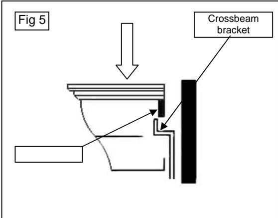
Run a thin line of cement on the wall and along the top edges of the legs and carefully lower the crossbeam into position locating the holding block onto the crossbeam bracket. Ease all joints together and review total alignment, taking care with corners and edges.
