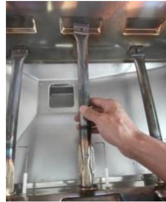
3. Remove LP (Liquid Propane) orifice with 6mm nut driver for each of the main burners, and replace with 1.77mm NG orifice by hand (4 main burners).
