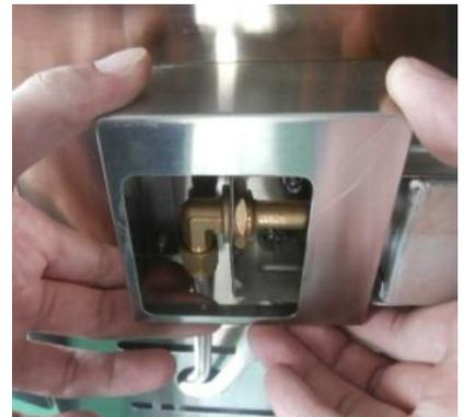
2. Remove the (Liquid Propane) orifice with 6mm wrench.
