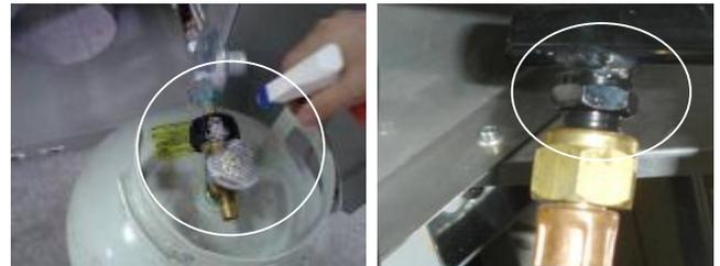
7. If you have a gas connection leak you cannot repair, turn gas OFF at supply tank, disconnect fuel line from your grill and call Canada: 800-648-5864, U.S.: 800-913-8999 or your gas supplier for repair assistance.
