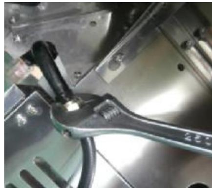
2. Install the NG (Natural Gas) regulator hose to the manifold and secure using a wrench. Tighten the NG regulator on the side panel with two 5/32\*10mm screws that pre-assemble on the NG regulator.
