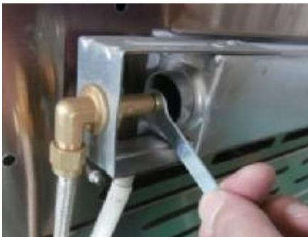
3. Replace with 1.84MM NG orifice with 6mm wrench. Then put rear baffle and screw back into the original position.
