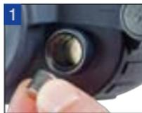
battery case by turning it counterclockwise. Exchange used round cell batteries with new ones.
