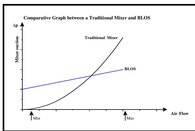
**the direction of the arrows)** is subjected to a pressure drop. The pressure differential created propagates on the two sides of the diaphragm by provoking a resulting upward force that produces the piston opening till the balance position is reached.
