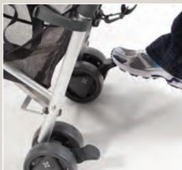
**TO SET BRAKE:** Press down each foot pedal to lock.
