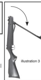
**BREAK BARREL AIR RIFLES** — With one hand grasp stock firmly behind trigger guard, avoiding contact with the trigger, and brace the butt end of the stock against your thigh. Grasp the barrel near the muzzle end, just behind the front sight. Pull downward and to the rear until it comes to a solid stop. You will hear a click indicating that the spring piston has been locked into position (see illustration 3).
