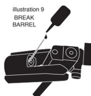
**CAUTION:** CHECK THE TIGHTNESS OF THE FRONT TRIGGER GUARD AND STOCK SCREWS BETWEEN, DURING, AND AFTER SHOOTING ACTIVITY. LOOSE SCREWS MAY CAUSE INJURY OR DEATH.
