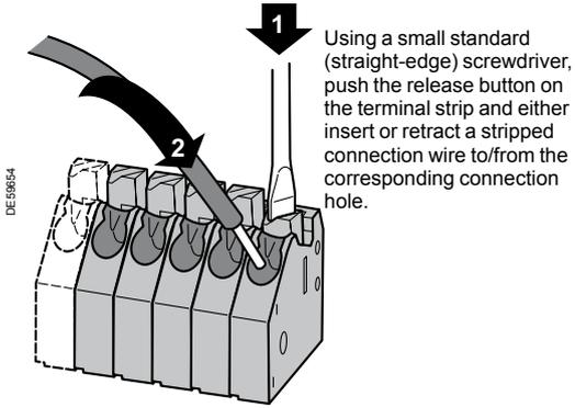
Using a small standard (straight-edge) screwdriver, push the release button on the terminal strip and either insert or retract a stripped connection wire to/from the corresponding connection hole.
