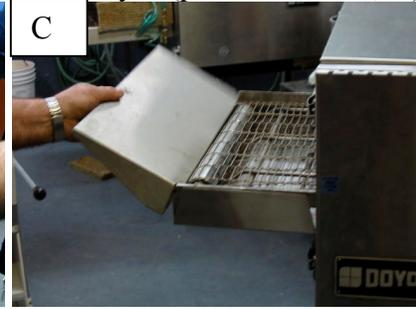
Pull out the conveyor motor cover (picture E & F).
