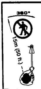
The operator of the machine must insure that no one comes within a 15 meter radius while working. When several operators are working within the same area a safety distance of at least 15 meters must be observed.
