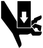
Pinch point hazard. Crimp ram operates at high speed and force and can cause severe personal injury. Keep all body parts away from moving parts of the tool during operation.
