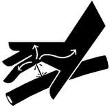
Hydraulic fluid under pressure. Do NOT use any part of your body to locate a hydraulic leak. Escaping fluid under pressure can cause severe injury or death. If injury results from escaping hydraulic fluid, seek immediate medical attention to avoid serious bodily injury.
