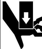
Pinch point hazard. Crimp ram operates at high speed and force and can cause severe personal injury. Keep all body parts away from moving parts of the tool during operation.
